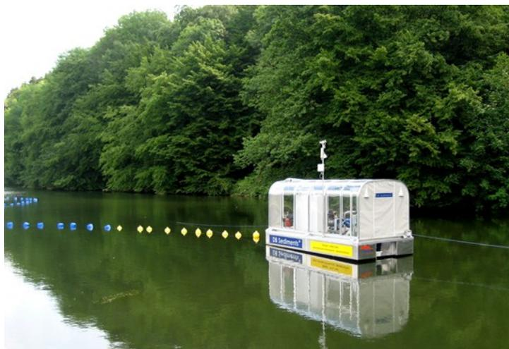
**Figure 3.1** Sediment transfer vessel “SediMover” (automatic, electrically driven, Type 101).
