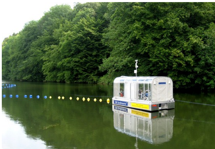
Figure 3.1 Sediment transfer vessel “SediMover” (automatic, electrically driven, Type 101).
