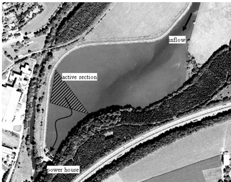
Figure 3.3 Sectional treatment of reservoir (Ehreshoven II reservoir/Germany).
